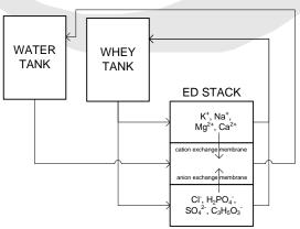
Fig. 1: Electrodialysis process scheme
