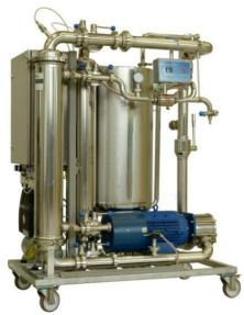
the unit makes itself backwash, chemical cleaning (CIP) and batch ending in case of need. We also offer a unit with two modules in version with a semi-automatic control — backwash is made automatically, but chemical cleaning is necessary to manage personal. Further it is possible to display the chart of filtrate flow trend in time. The unit ensures easy sanitation of whole system.
