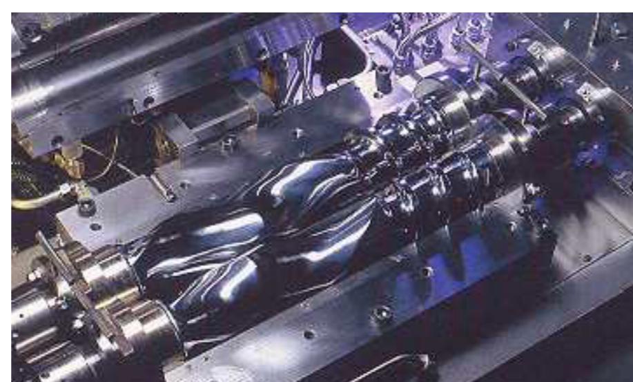
Picture 2: Non intermeshing rotors for CM
