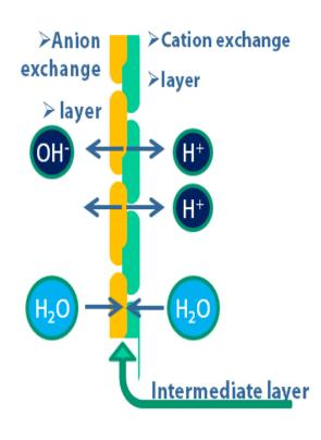
➢Bipolar membrane is a cation-exchange membrane combined together with an anion-exchange membrane, through an intermediate layer (the "junction" layer). This membrane arrangement placed in a high density electric field enhances dissociation (splitting) of water into H<sup>+</sup> and OH<sup>−</sup> ions.
