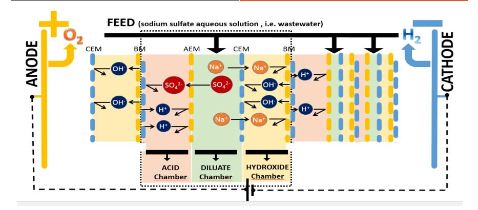
Three-chamber arrangement - production of acid and base at the same time, higher current efficiency can achieve higher concentrations of products suitable for processing salts of strong acids or bases (Na2SO4). Concentration of the resulting solutions is about 4% w / w.
