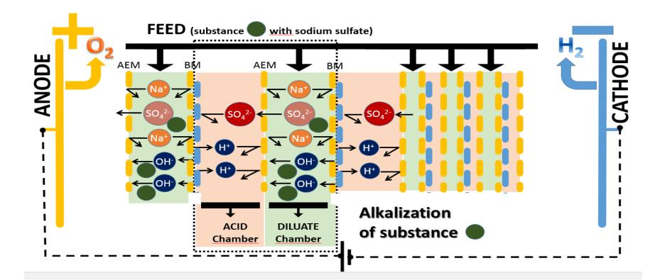
Two-circuit arrangement - easier, production of either acid or alkali, less electrical resistance, higher concentrations of H + and OH- at low concentrations, suitable for the treatment of salts of weak acids or alkalis, for acid and alkaline purification of salts and alkalis
