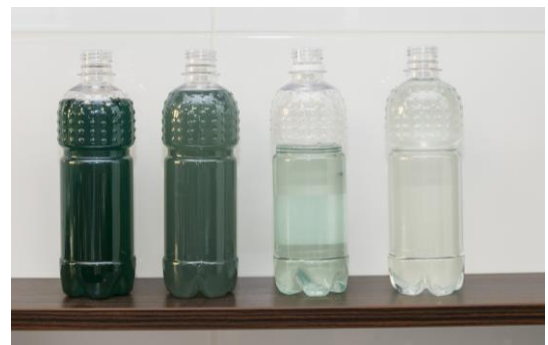
From feed to product (glycol mixture in different phases of purification)
